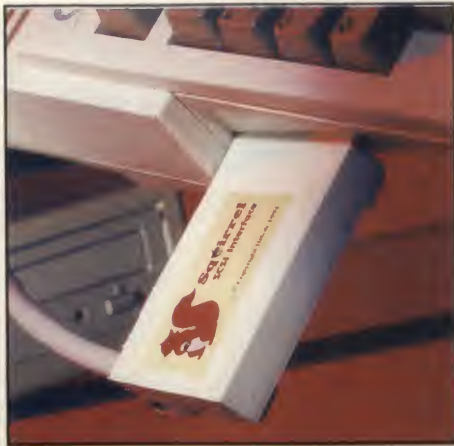
The Squirrel, and now the Surf Squirrel, are almost a de facto standard for A1200 SCSI connections.
